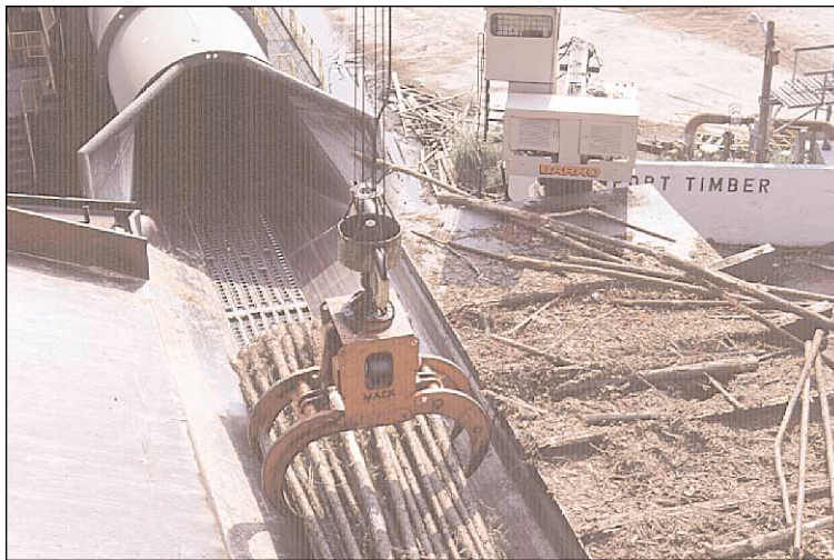
The debarking drum is fed by a KoneWood™ Powerfeed™ infeed system, with a Newport Timber-specified dual zone drive.
