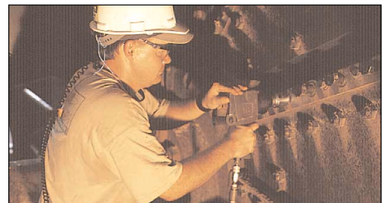
A view of the Andritz KoneWood™ HH902 chipper, taken during a knife change.
