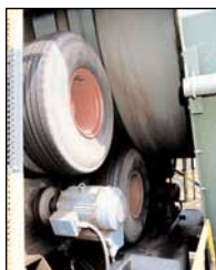
The debarking drum's rubber tire support and drive system makes it an economical alternative to traditionally-designed drums.
